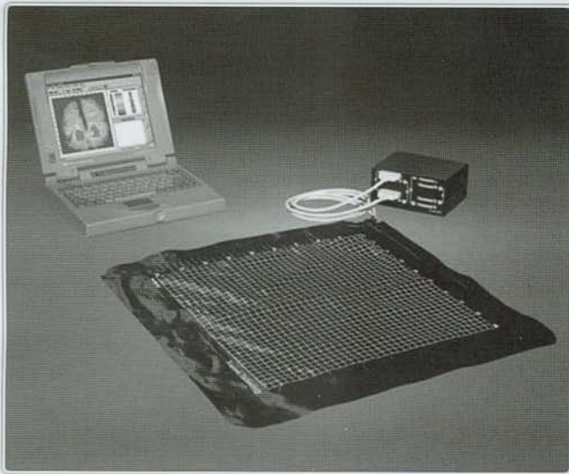
Figure 17. The Xsensor Pressure Mapping System. This unique method and clinical tool is used to assist in measuring interface pressures that occur between patients and their contact surfaces. The measuring device is a soft, pliable mapping pad that conforms to the surface and user.
