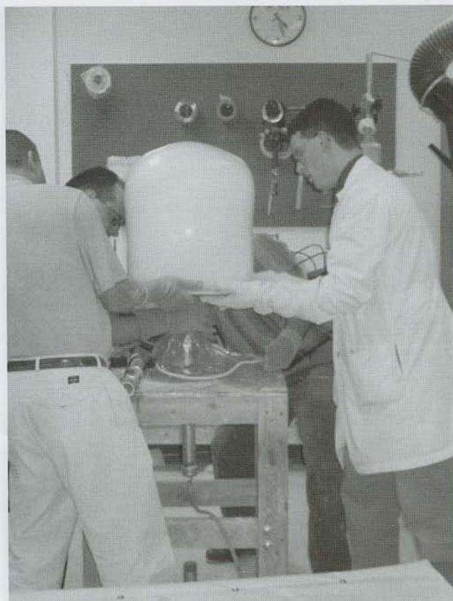
Figure 9. Once the positive mold has been rectified, a high-density Plastazote filler is formed directly on a plaster model and then the rigid outer frame is blister-formed using ¼-inch high-density polyethylene.
